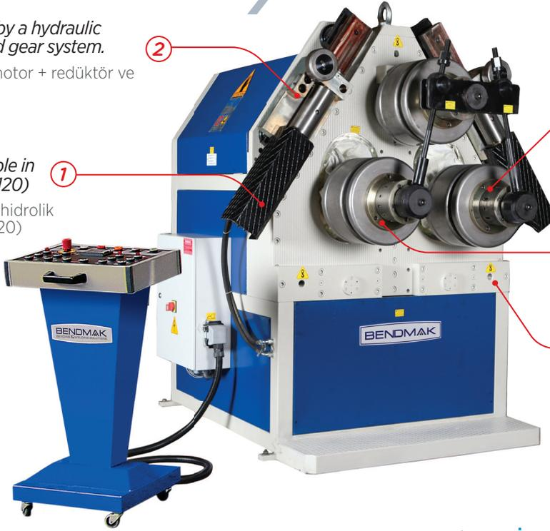
3 Bottom rolls hydraulically moveable up and down
