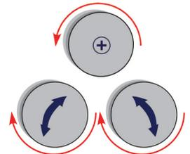
Optional guide rolls hydraulically adjustable in two directions
