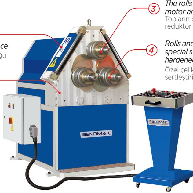
**The rolls are driven by a hydraulic motor and gear system**
